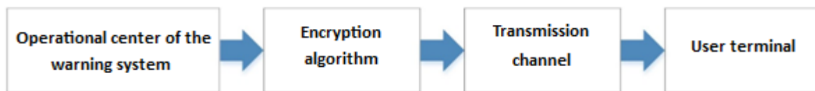
Figure 2: Basic elements of a system for positionally forced transmitting of information
